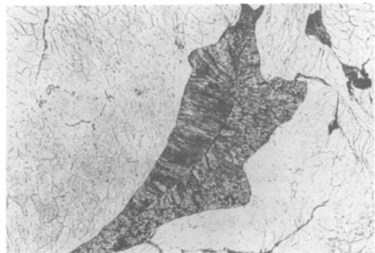
Figure 11 A rare example ( \times 300 ) where columnar-like, "as-cast" grains were detected in the melted zone.
